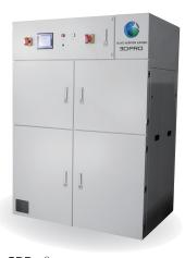
Provides the ideal low oxygen and moisture environment for metal powder storage before processing.
