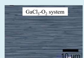
Fig.14 Optical microscopy image of  $\beta$ -Ga<sub>2</sub>O<sub>3</sub> surfaces after HVPE growth.
