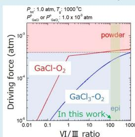
Fig.12 Comparison of the  $\Delta P_{\text{Ga}_2\text{O}_3}$  in GaCl-O<sub>2</sub>-N<sub>2</sub> and GaCl<sub>3</sub>-O<sub>2</sub>-N<sub>2</sub> systems [2].
