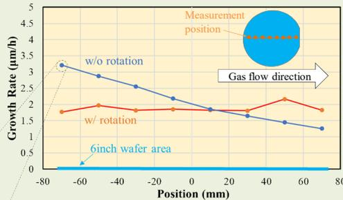
Fig.11 Thickness distribution of  $\beta$ -Ga<sub>2</sub>O<sub>3</sub> layer grown on a 6-inch sapphire wafer (along the gas flow direction).
