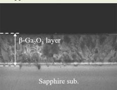
Fig.10 Cross-sectional SEM image of  $\beta$ -Ga<sub>2</sub>O<sub>3</sub> layer grown on a 6-inch sapphire wafer.
