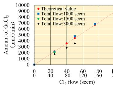
Fig.7 Relationship between Cl<sub>2</sub> flow rate and amount of GaCl<sub>3</sub> generation\*.
