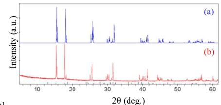
Fig.8 XRD data of solidified powder in a quartz trap\*. (a) Calculated GaCl<sub>3</sub> data from crystal structure [1]. (b) Measurement result of powder trapped in quartz trap.
