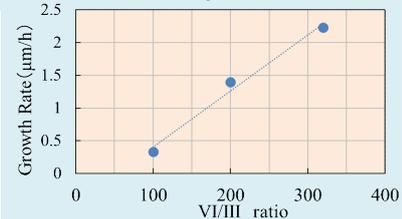
Fig.13 Growth rate of Ga<sub>2</sub>O<sub>3</sub> as a function of VI/III ratio.
