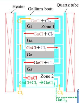
Fig.6 Cross sectional view of GaCl<sub>3</sub> generator (prototype).
