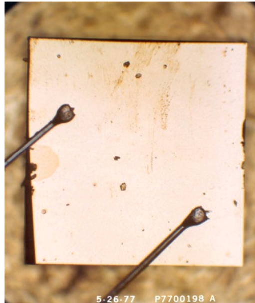
FIG. 8. Optical micrograph of the first MOCVD AlGaAs-GaAs broad-area DH laser diode taken on May 26, 1977. The device size was 800 \times 800 \mu\text{m}^2 and was mounted n -side down, and the two visible wire bonds were made to the p -GaAs:Zn contact layer. This chip had four cleaved Fabry-Perot facets. This device was operated under pulsed conditions at 300 K a few days before this photograph was taken on May 26, 1977.
