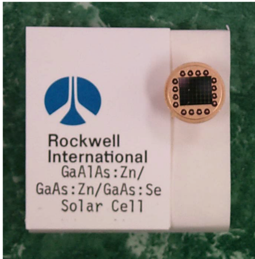
FIG. 6. Photograph of one of the first AlGaAs-GaAs “window” solar cells grown by MOCVD in 1977. The longer dimension of the device is \sim 1 cm. A simple “grid” contact pattern was used for this device. We subsequently developed a 1 \times 1 cm 2 device with an improved the top ohmic contact design for higher efficiency.
