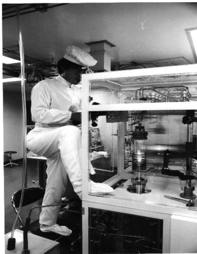
FIG. 25. Photograph of Hiroshi Amano working on the "home-made" III-N "MOCVD reactor in the Nagoya University MOCVD cleanroom in 1984. Compliments of Professor Hiroshi Amano. Photograph taken by Professor Kazumasa Hiramatsu. Used with permission of Professor Hiramatsu (Ref. 204).
